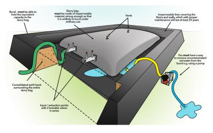
Figure 17.3. Earth banked slurry bag.
