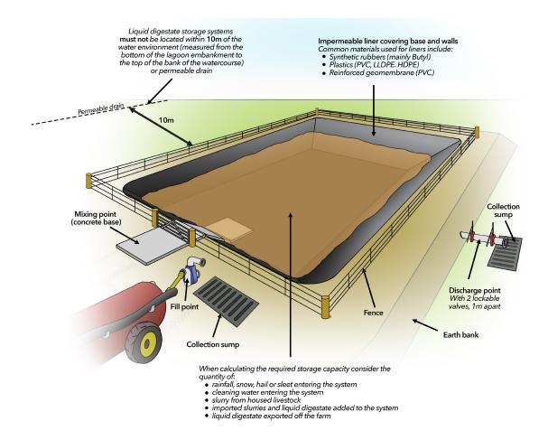
Figure 17.1 Anaerobic digestate storage lagoon.
